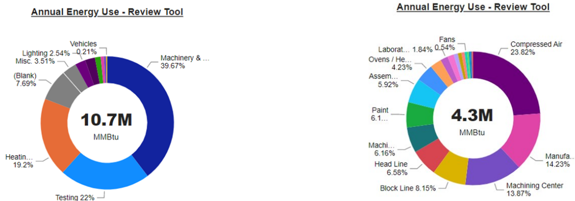
Figure 2: Summary of all site SEUs by % of energy used. Figure 3: Expanded Machinery & Equipment SEUs
